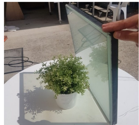
Switchglass ON 75% light passing through glass
