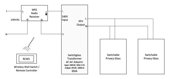
Switchglass 65VAC Transformer (240VAC to 65VAC) (130 x 90 x 70mm): 1 required per switchable area up to 5m<sup>2</sup>. PLEASE NOTE: The Transformer has a built-in fuse and must be located in an accessible position.
