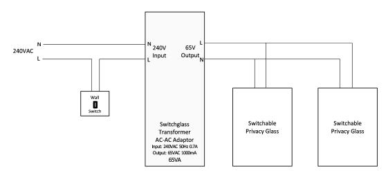
Switchglass 65VAC Transformer (240VAC to 65VAC) (130 x 90 x 70mm): 1 required per switchable area up to 5m<sup>2</sup>. PLEASE NOTE: The Transformer has a built-in fuse and must be located in an accessible position.
