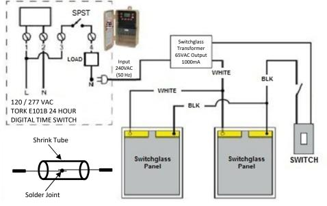
All connections must be soldered and sealed with shrink tubing. Wires can be extended with 18 AWG wires.
