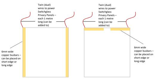
NOTE: Edges where the busbars are placed must be covered by minimum 12mm (recommend 18mm)
