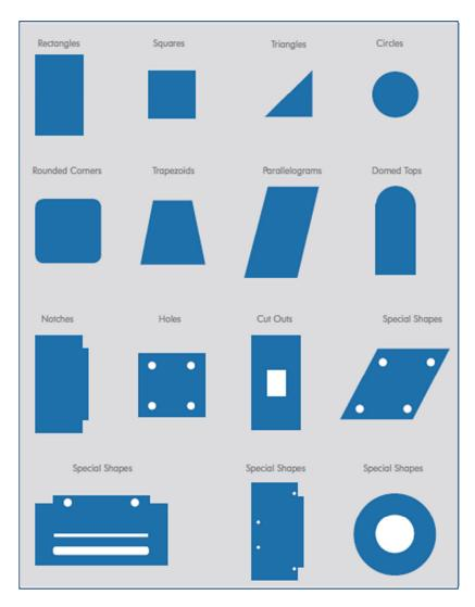
Clear, non-switchable areas, very small bubbles and/or visual distortion may be present around notches/holes and cut-outs. Therefore customers must allow for coverage of 10mm all around notches/holes and cut-outs.
